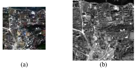
Fig. 6. Input QuickBird images. (a) Degraded MS image at an 11.2-m spatial resolution. (b) Degraded PAN image at a 2.8-m spatial resolution.
